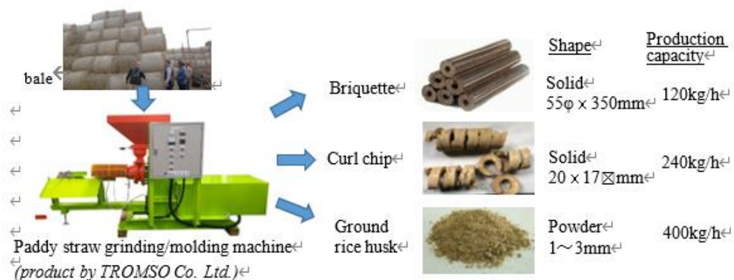
Figure 4-1 Biomass solid fuel conversion device and grinding production
