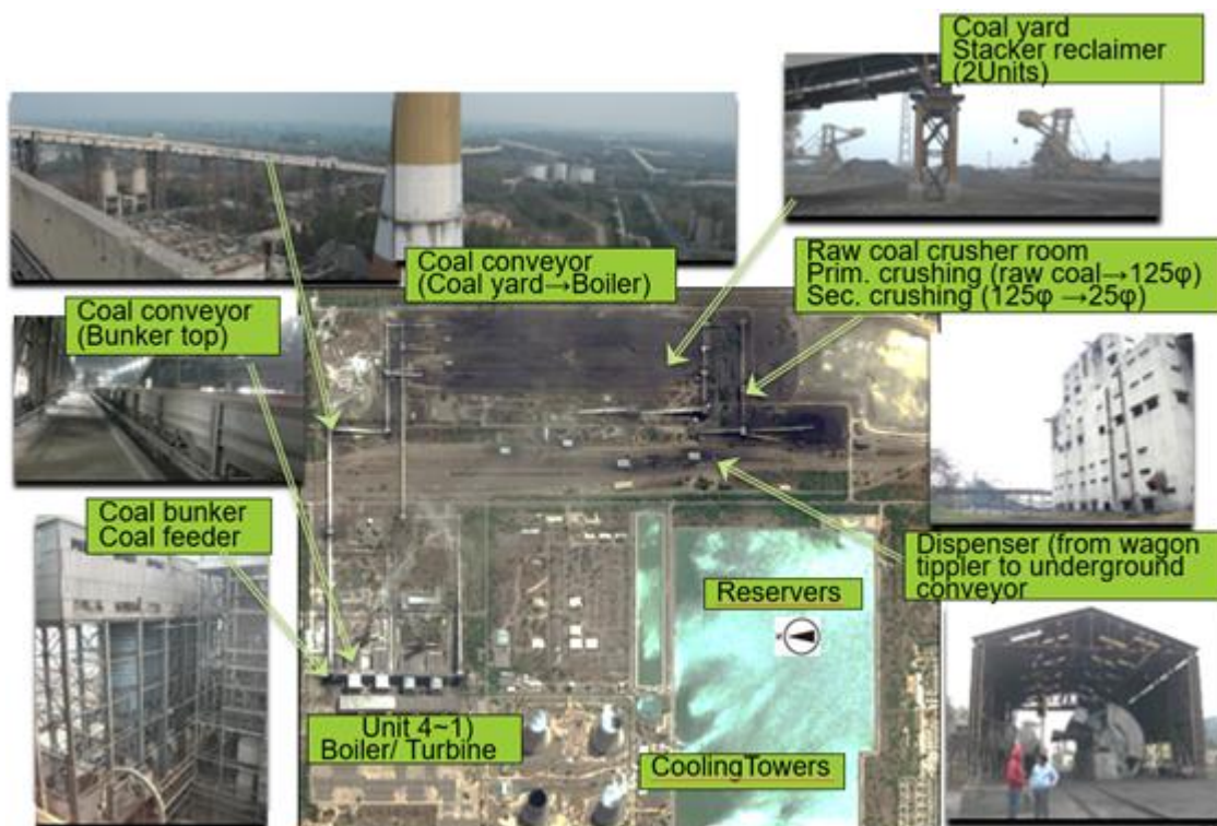
Figure 3-3 Unit layout and main facilities of GHTP
