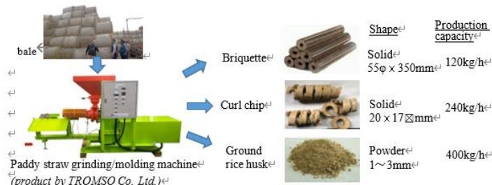
Figure 3-7 Biomass solid fuel conversion device
