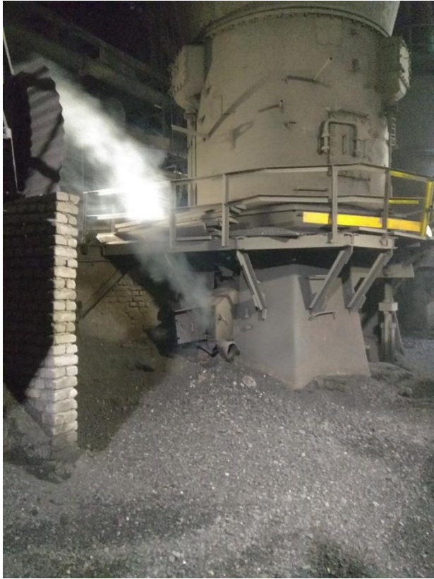
Pulverize fuel leakage from Mills
