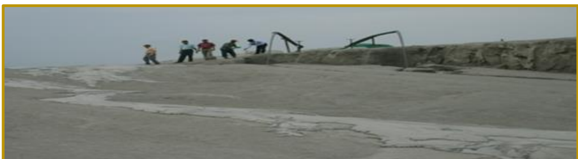
Figure 4: High Concentration Slurry Flowing on Slopes which dries out by the time it travels 30-40 m from the source
