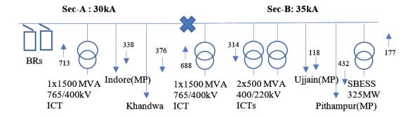
No issues were observed under 'n-1' of 765/400 kV ICT in either section.
