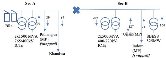
Among the three alternatives, power flow is balanced in both the sections in **Alternative-4** i.e. closing bus sectionaliser does not lead to significant flow from one
