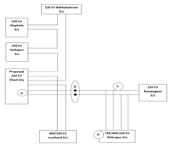
Point A – Point B = 13.5 km Proposed D/C line Point C – Point D = 5 km proposed M/C line
