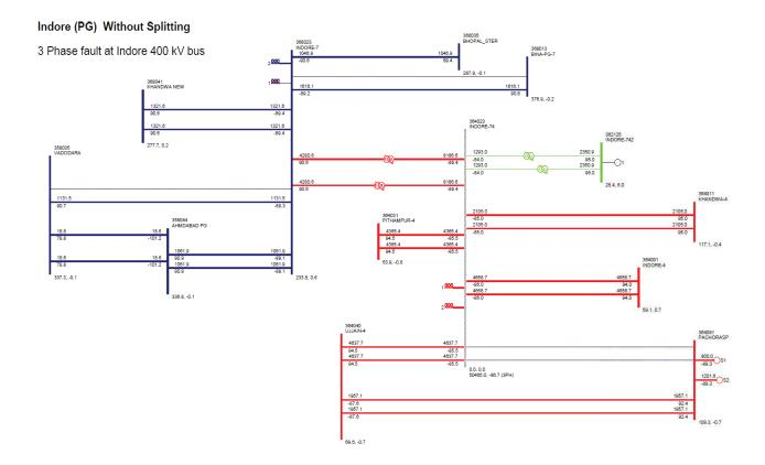
Accordingly, System study was carried out by CTU for 2022-23 time frame for High RE and Low RE scenarios to control the high fault level at Indore(PG) S/s keeping in view the fact that 765/400 kV ICTs, Indore (MP), Ujjain (MP) and Pithampur (MP) feeders are the major SC Fault contributors at Indore 400 kV (PG) S/s. Study results for various configurations are enclosed at Annexure-XVII.
