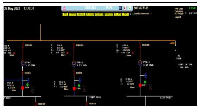
Figure 8. SLD on SCADA display
