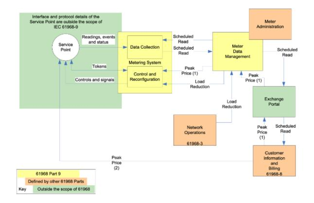
Key IEC 61968-9 Interfaces relevant for the scope are meter reading and control messages as below. Detail of each interface request and response can be referred in IEC 61968-9 document.
