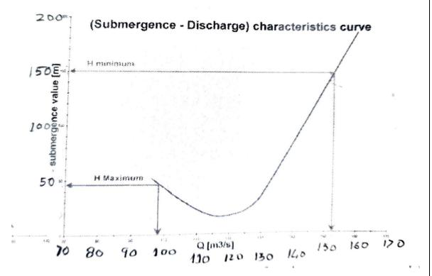
As in Tehri PSP, head range is very large which implies that the pump operates while NPSH becomes high at extreme heads. Although, lower value of submergence could be obtained by specific ways of closing of wicket gates, but this would mean dissipation of energy in the machine at low heads and then resulting the sharp decrease of efficiency, a bigger runner and also risk of excessive vibration zone and thus was not accepted.
