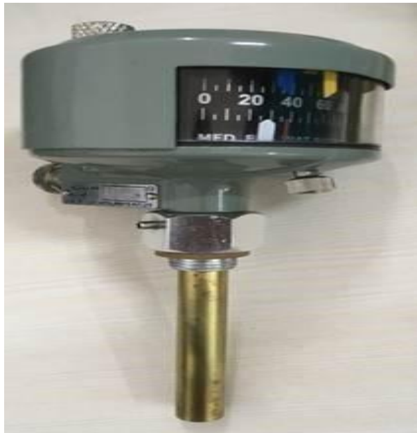
Fig. 3: Oil Temperature Indicator (OTI)
