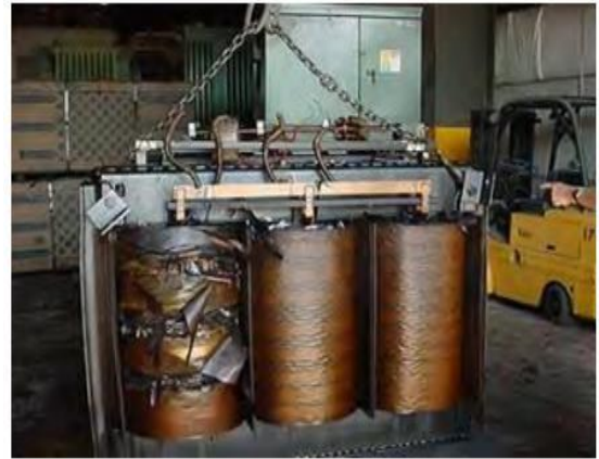
Figure 2: Inter-Turn Faults due to poor insulating material
