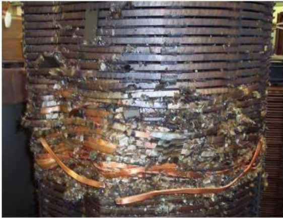
Figure 2: Inter-Turn Faults due to poor insulating material
