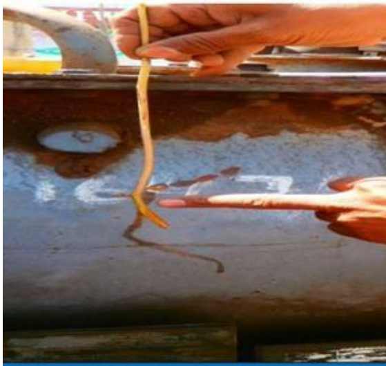
Figure 11: Low Oil Level
