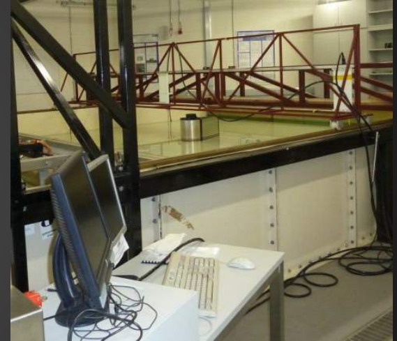
NUI Galway tidal basin with GKInetic 1/40 scale prototype
