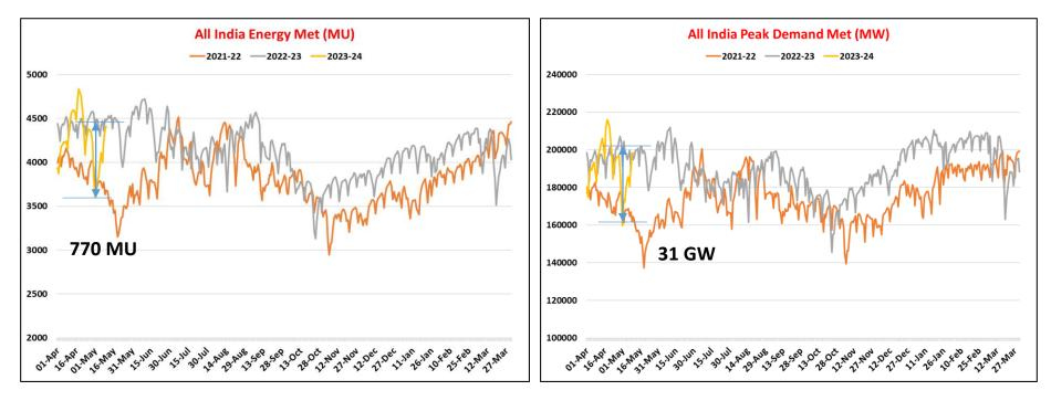
Significant increase in both Maximum Demand and Energy Met in Q4 of FY 2022-23 & Q-1 of FY 2023-24 as compared to same quarter of previous year. However, Inclement weather and widespread rains across the country has led to load crash in the start of May'23
