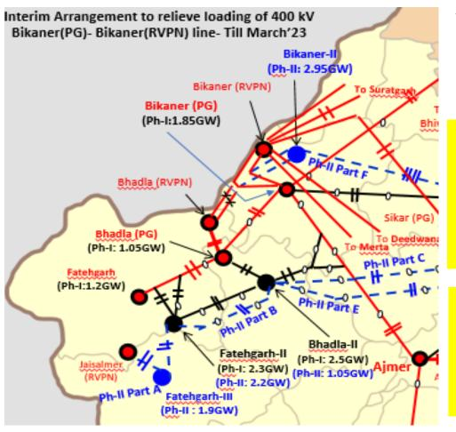
The Phase-I transmission system has mostly been commissioned whereas transmission elements part of Phase-II transmission scheme are yet to be commissioned. (Currently, 3200 MW RE in Rajasthan is being evacuated through STOA)
