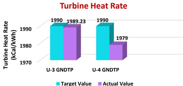
**Fig. 4.18:** Heat Rate values (Target vs. Actual) of GNDTP Unit-3&4 Turbine
