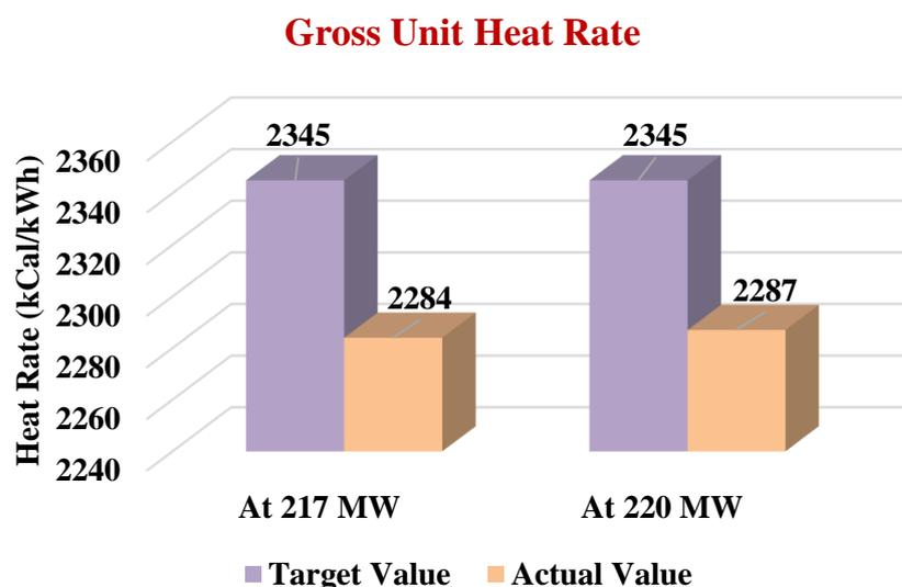
**Fig. 4.19:** Gross Unit Heat Rate values (Target vs. Actual) of Unit-5 of Bandel TPS
