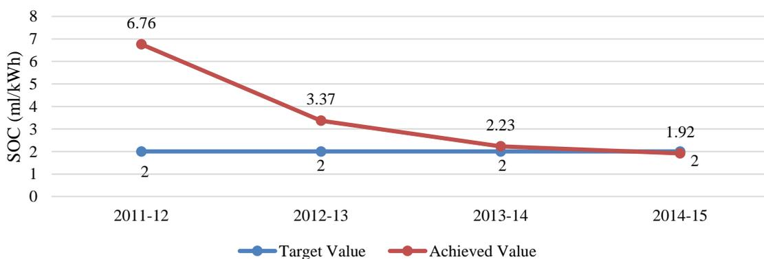
**Fig 4.12:** Amarkantak TPS SOC values (Target vs. Achieved) after R&M for unit-1 & 2
