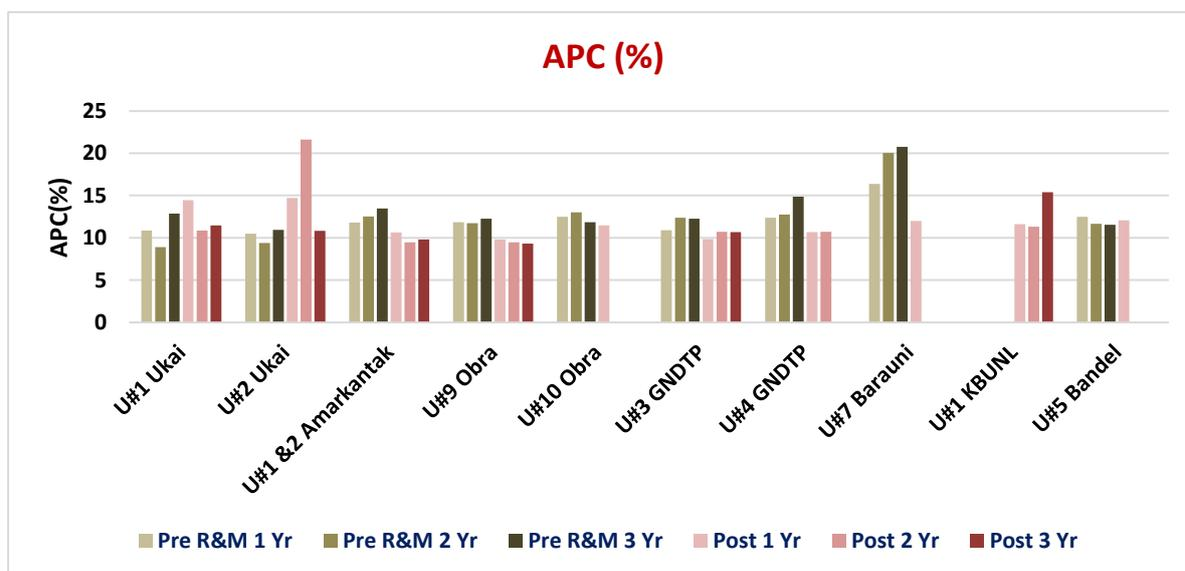
**Fig. 4.4:** Comparative Analysis of Auxiliary Power Consumption before and after R&M
