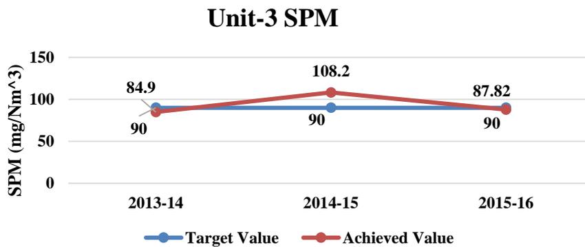
**Fig. 4.17:** GNDTP Unit-3 SPM values (Target vs. Actual) after R&M
