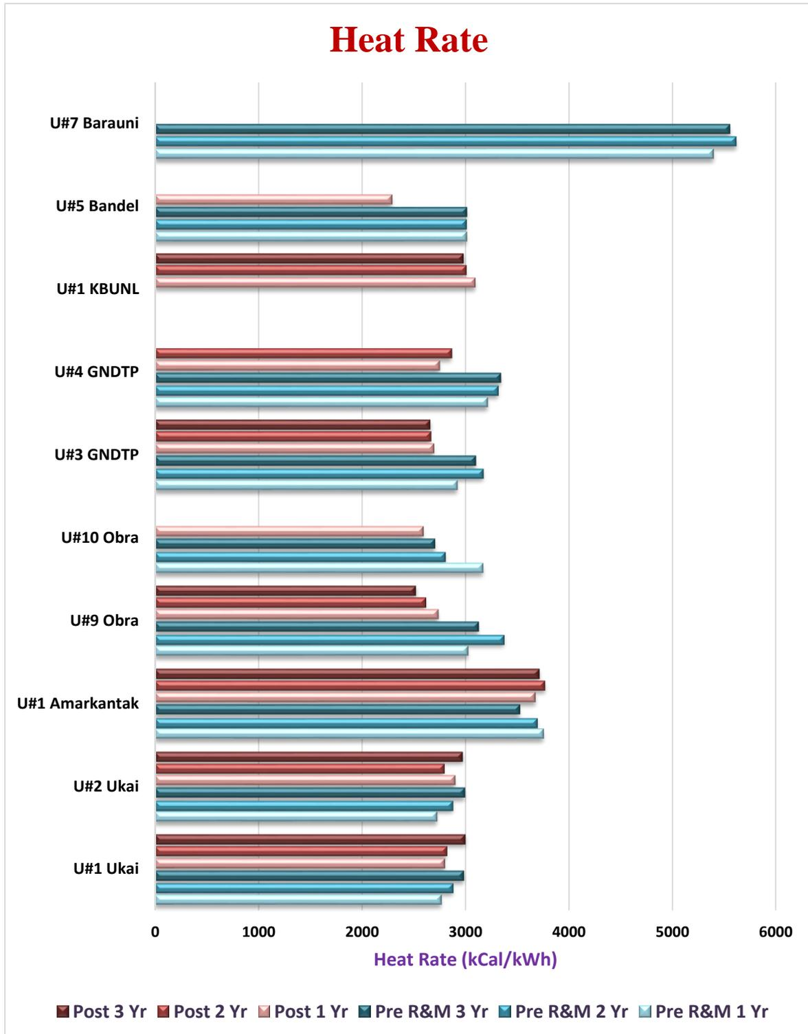
**Fig. 4.7:** Comparative Analysis of Heat Rate Pre and Post R&M
