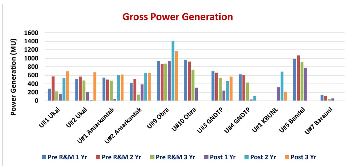
**Fig. 4.2:** Comparative Analysis of Gross Power Generation before and after R&M
