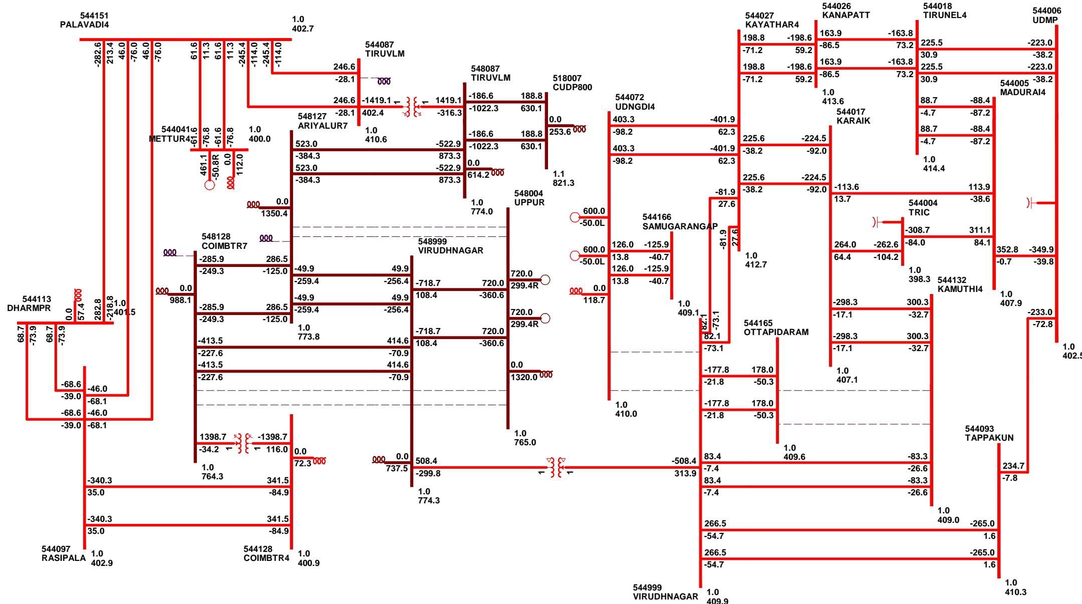
LOAD FLOW STUDY - UPPUR 2X800 MW THERMAL POWER PROJECT
