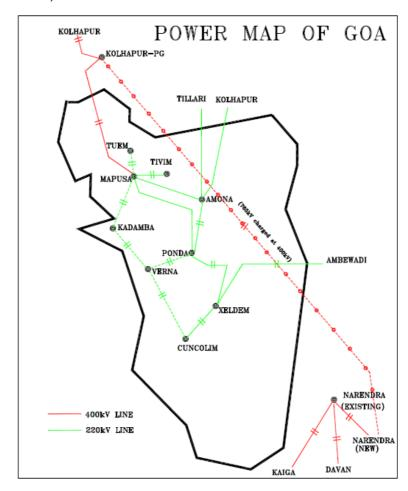
To improve the reliability and power supply situation in Goa, an additional 400 kV in feed to Goa proposed. **Two alternatives** have been explored as given below:
