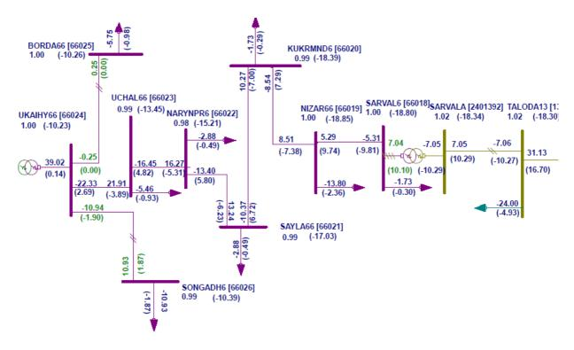
c) With 132 kV interconnection between Taloda (MSETCL) and Sarvala(GETCO) substations and Naranpura-Sayla 66 kV S/C line kept
