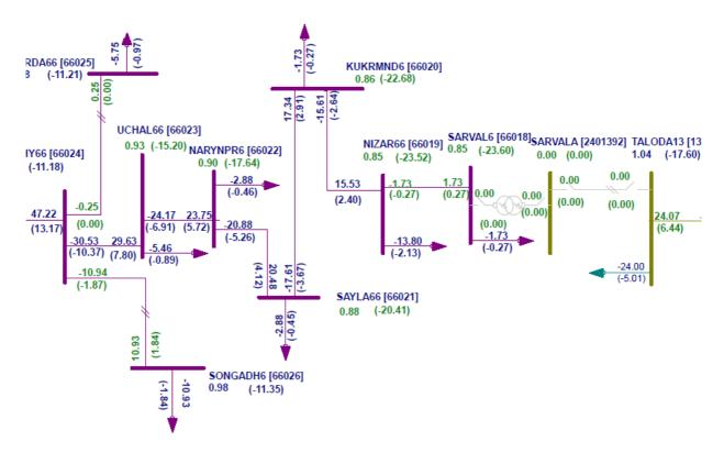
b) With 132 kV interconnection between Taloda (MSETCL) and Sarvala(GETCO) substations. The studies shows there is power flow of about 23 MW on Ukai- Uchal-Naranpura-Sayla-Kukarmunda-Nizar 66 kV S/C line and about 7 MW power flow from Maharastra to Gujarat on the Taloda-Sarvala 132 kV D/C line. The voltages observed on the 5 nos. of 66 kV substations (Uchal, Naranpura, Sayla, Kukarmunda and Nizar) is around 1 p.u.
