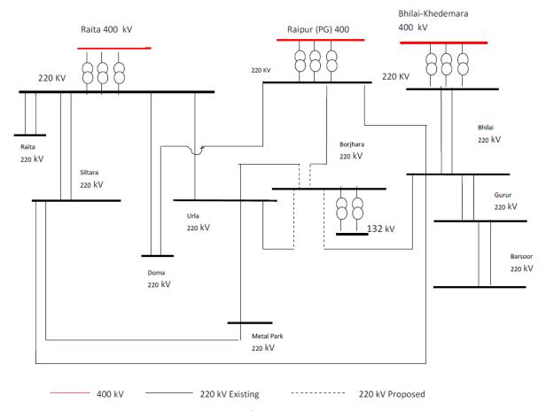
6.2 The above proposal involves LILO of 220 kV line emanating from inter state 400/220 kV substation, therefore it is put for the approval of the standing committee. The power flow on these lines is tabulated below:
