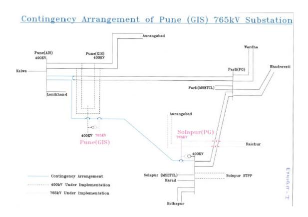
4.3 The studies carried out by POWERGRID with 1250 MW export from WR to SR over Sholapur- Raichur 765 kV D/C line is enclosed as Annexure-1. Pune (GIS) – Sholapur 765kV S/C line at 400kV provides an additional in feed to Sholapur which helps in power transfer to SR in case of outage of one circuit of Parli – Sholapur 400 kV S/C line.
