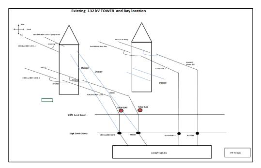
30.2 In view of the above, it was proposed to rearrange lines in four line bays (2 no. line bays of POWERGRID and 2 no. line bays of E&P Dept., Govt. of Sikkim) such that there are no clearance issues. For this, E&P Dept., Govt. of Sikkim would use one bay of POWERGRID for termination of its Chuzachen line and accordingly POWERGRID would utilise one of the bays of E&P Dept., Govt. of Sikkim for termination of Melli line. The revised arrangement is shown below:
