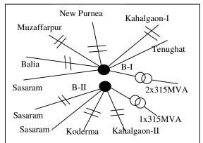
In the Biharsharif substation, splitting of substation along with swapping of Purnea bays(1 & 2) with Sasaram bays (3 & 4) (both are quad lines) and Kahalgaon#1 bay with Sasaram#1 bay would be required.
