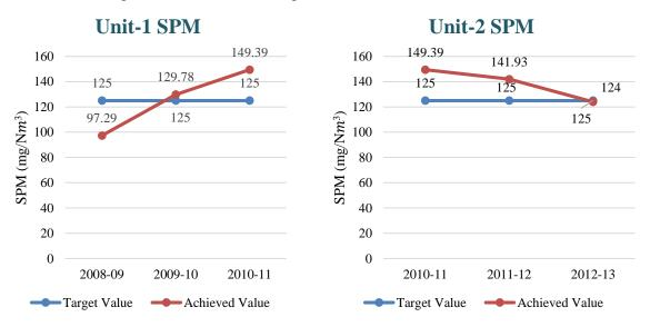
Fig. 4.10: Ukai Unit-1&2 SPM values (Target vs. Achieved) after R&M
