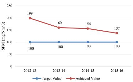
Fig. 4.15: Obra Unit-9 SPM values (Target vs. Actual) after R&M
