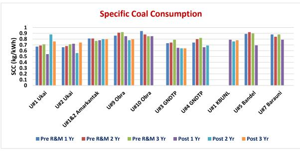
Fig. 4.6: Comparative Analysis of SCC Pre and Post R&M
