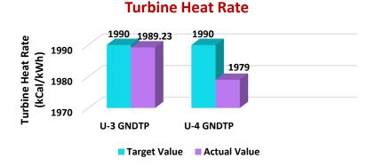
Fig. 4.18: Heat Rate values (Target vs. Actual) of GNDTP Unit-3&4 Turbine
