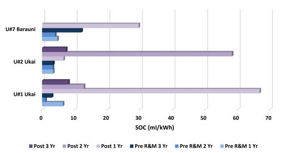
Fig. 4.5 (b): Comparative Analysis of SOC Pre and Post R&M
