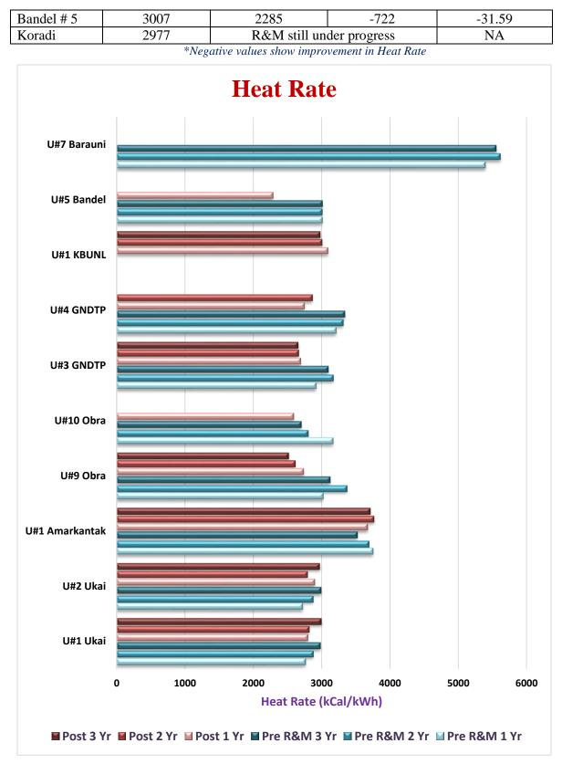
Fig. 4.7: Comparative Analysis of Heat Rate Pre and Post R&M
