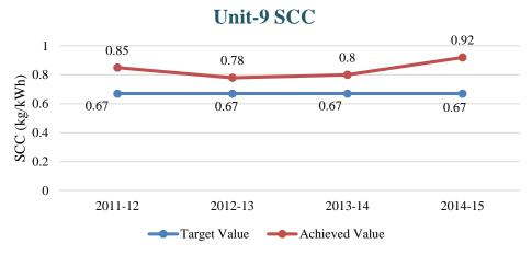
Fig. 4.14: Obra Unit-9 Specific Coal Consumption values (Target vs. Actual) after R&M
