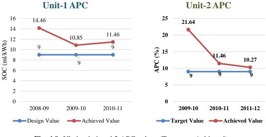
Fig. 4.9: Ukai unit-1 and 2 APC values (Target vs. Achieved) after R&M
