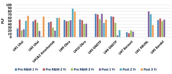
Fig. 4.3: Comparative Analysis of PLF before and after R&M
