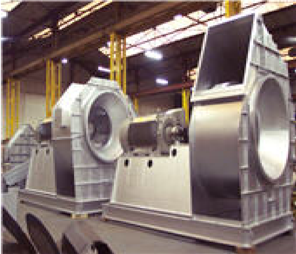
Power Station Fan
