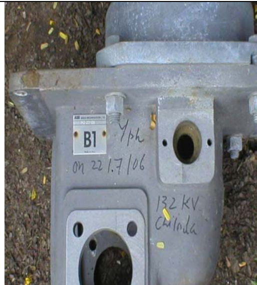
Exhibit-6 Broken metallic part disengaged from common driving rod
