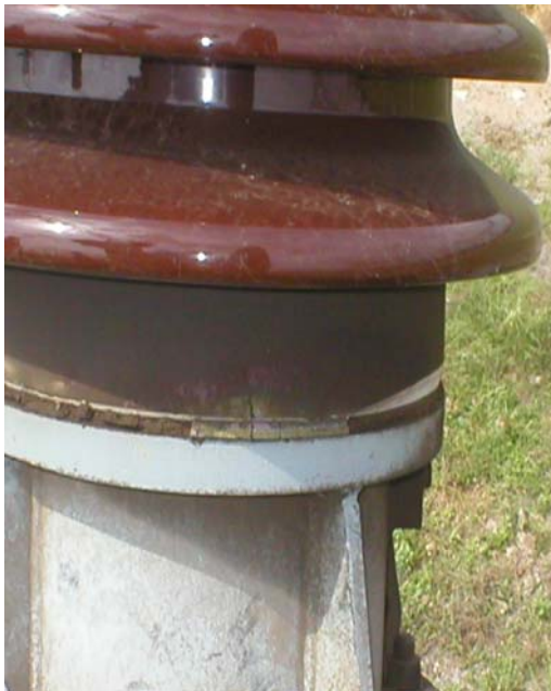
Exhibit-5 Displacement of bushing from cemented portion
