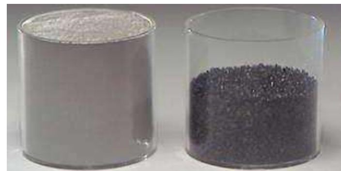
Fly-ash (Conventional Boiler) Glassy Molten Slag (IGCC) Approx. 60% decrease in volume
