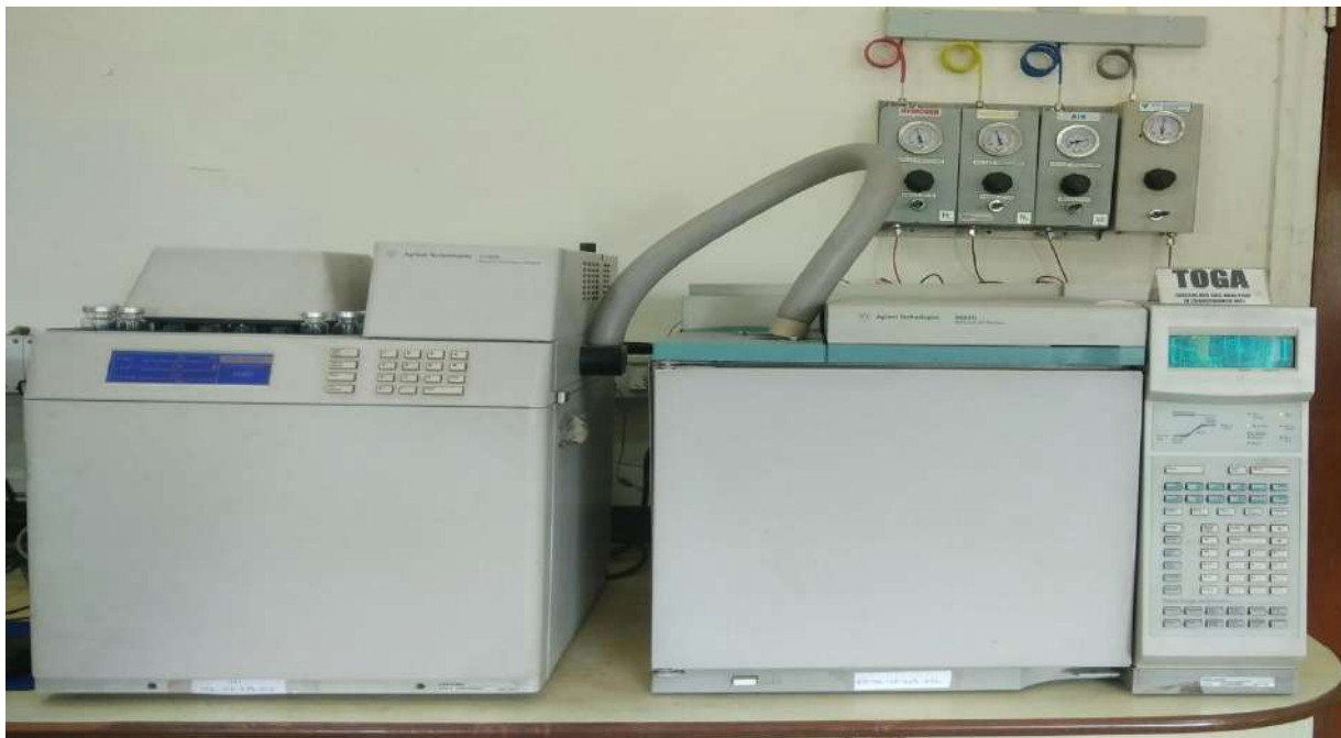
Fig 5 DGA equipment for stray gassing as per ASTM D 7150.
