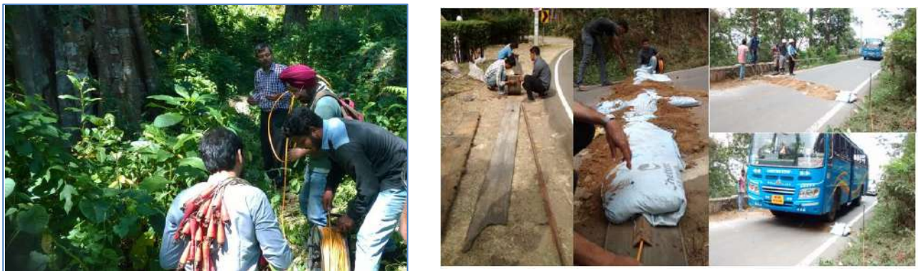
Fig. 4: Laying of imaging cables and arrangement for safe passage of imaging cable across NH-49
