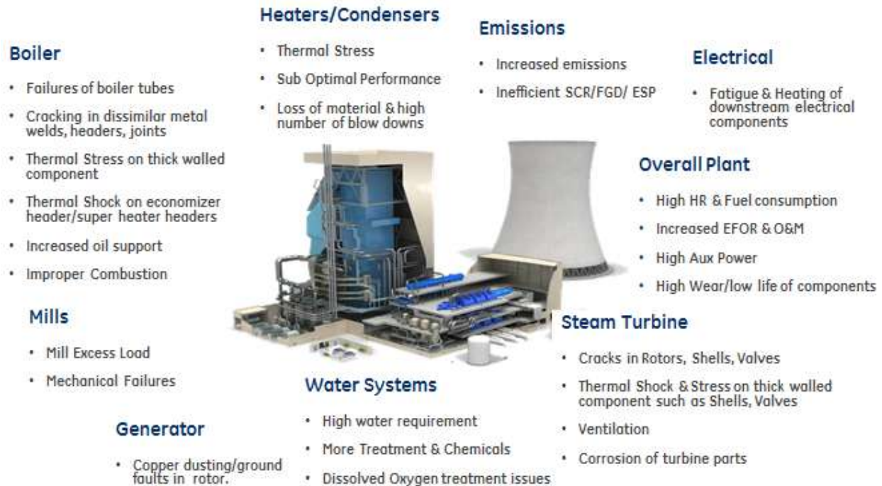
Figure-5: Overview of equipment/ system side challenges
