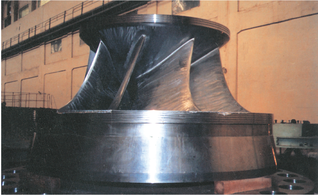
New Turbine Runner of Unit No. 3 of Burla Power House of Hirakud Power System being replaced for RIM & U Works.
