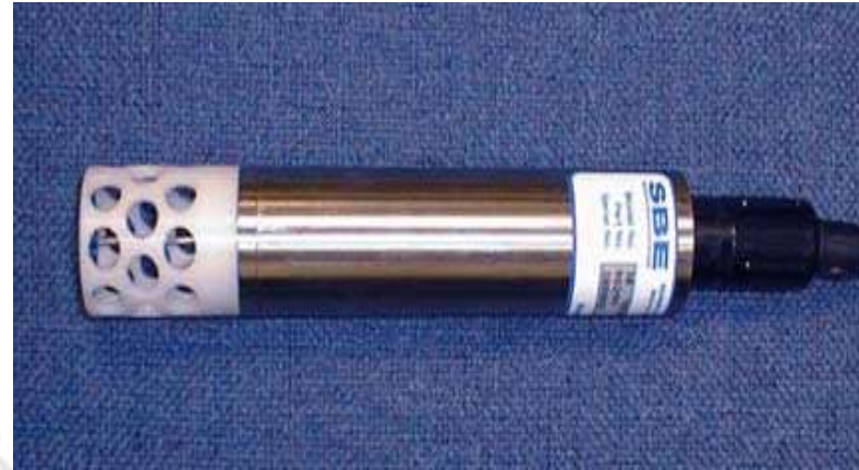
SBE 38 Seabird Thermometer
