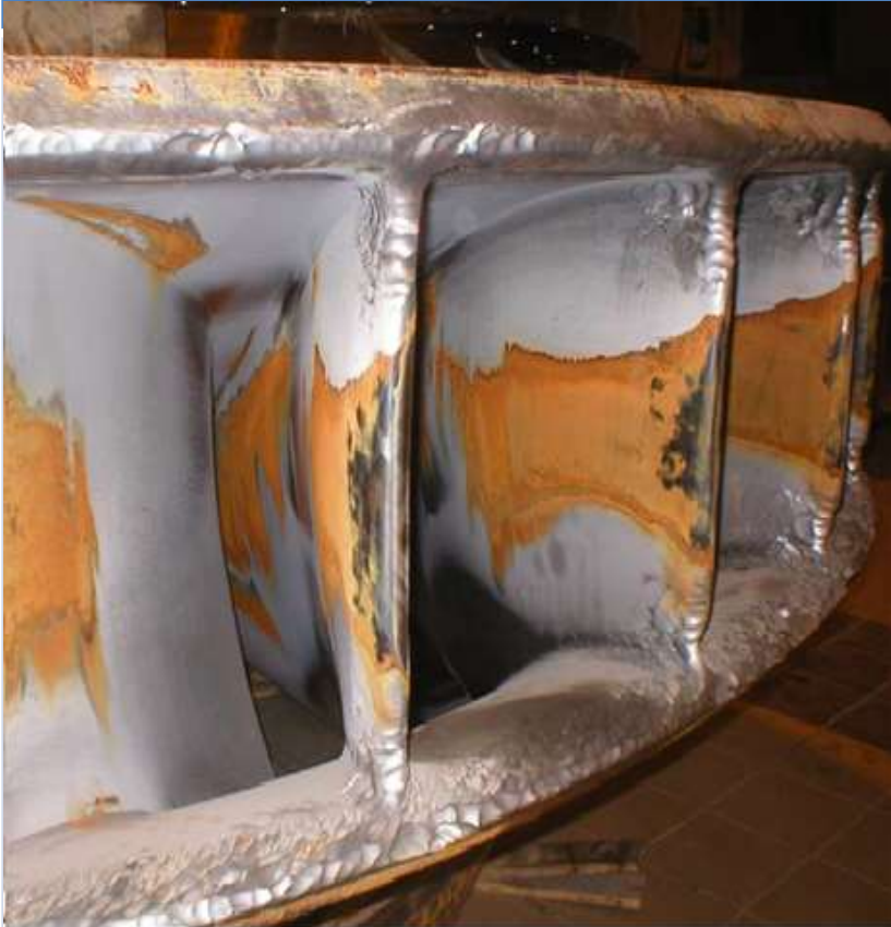
uncoated 16:5 runner after one year of operation
