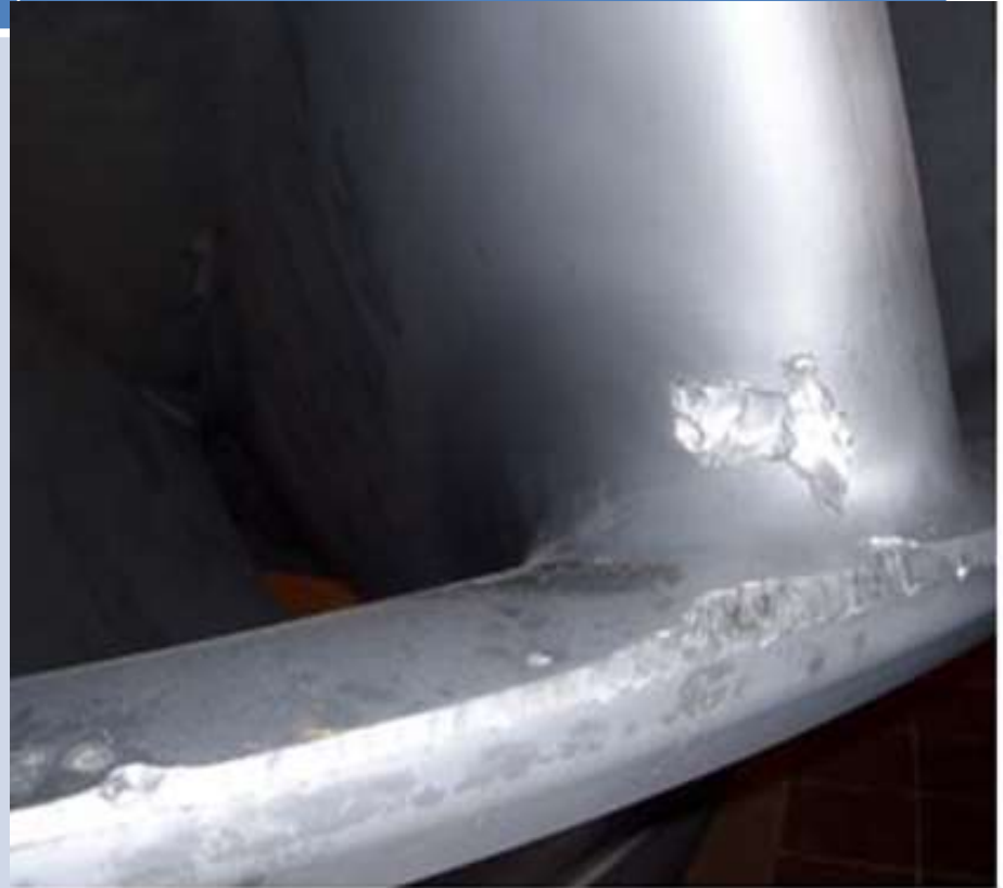
coated 13:4 runner after one year of operation
