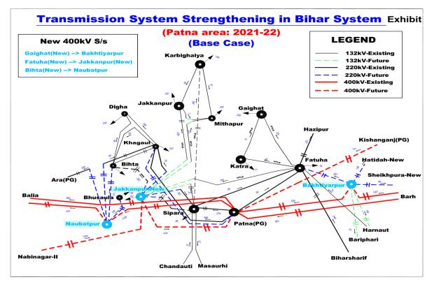
12.7 After deliberations, members agree for establishment of 3 no. 400kV GIS substations at Naubatpur, Bakhtiyarpur and Jakkanpur in place of Bihta, Gaighat and Fatuha respectively along with down-linking 220kV & 132kV works and other transmission works mentioned above as **Phase-IV - Part-II** transmission works to be implemented by BSPTCL as intra-state transmission works.
