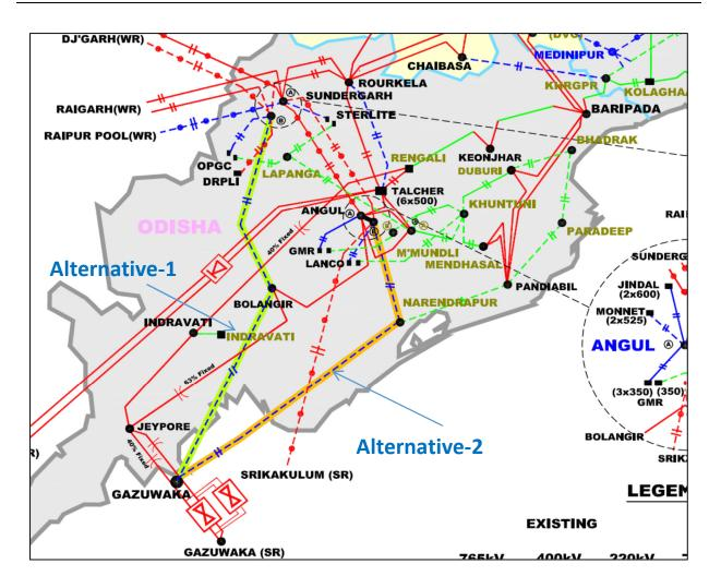
Jeypore S/s is fed from two 400kV lines viz. Angul/Bolangir – Jeypore and Indravati – Jeypore 400kV S/c lines (ACSR Twin Moose). Both lines have been constructed with thermal capacity of 874MVA. N-1 of any of these lines limits the power feed to Jeypore and Gazuwaka substations, thereby limiting the full utilisation of Gazuwaka HVDC.
