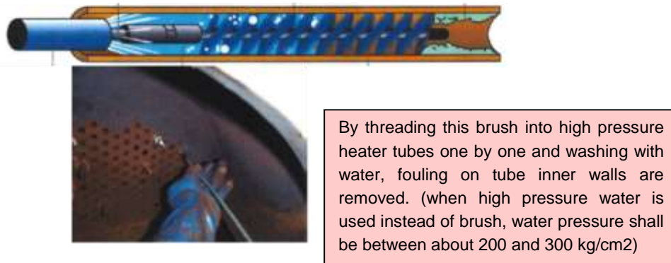
Figure 3-4 Brush dedicated to water-jet cleaning of high-pressure heater
