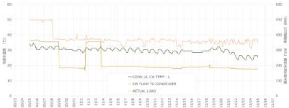
Figure 2-8 Record of the No. 1 Unit condenser cooling water temperature, flow and generator output
