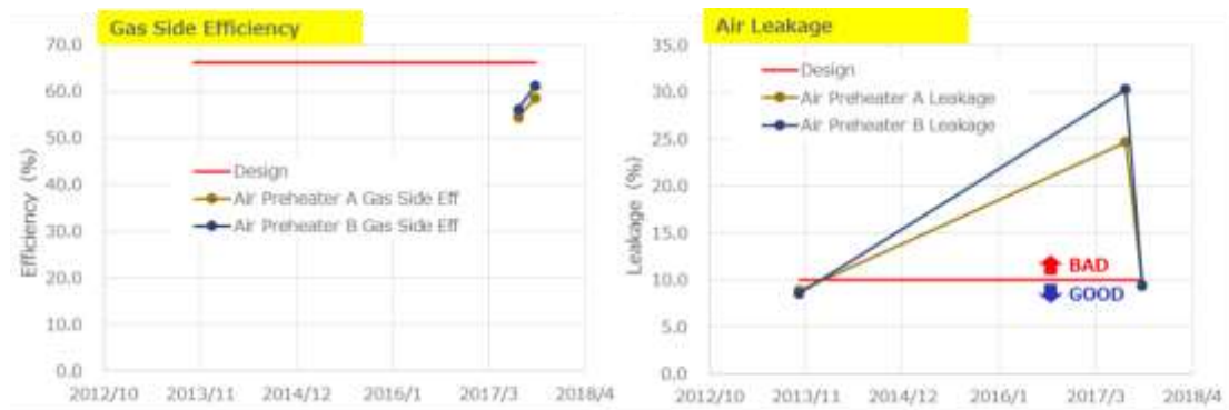
Figure 2-22 Transition and comparison with the design value of AH temperature efficiency and air leakage ratio
