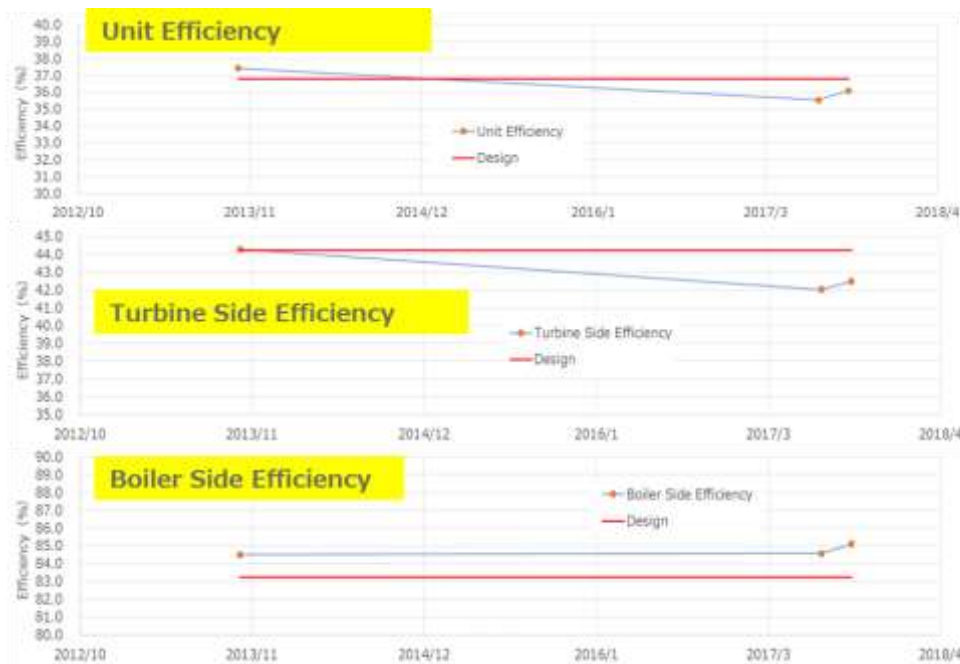
Figure 2-12 Actual performance and design value of the entire unit, turbine and boiler
