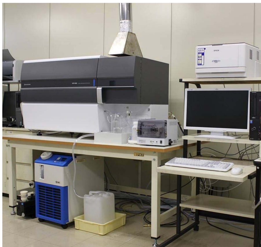
Figure 3.3-3 Appearance of ICP emission spectrometer
