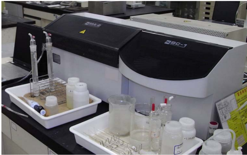
Figure 7.2. Hg analyzer (Nippon Instruments Corporation/MA-2000)
