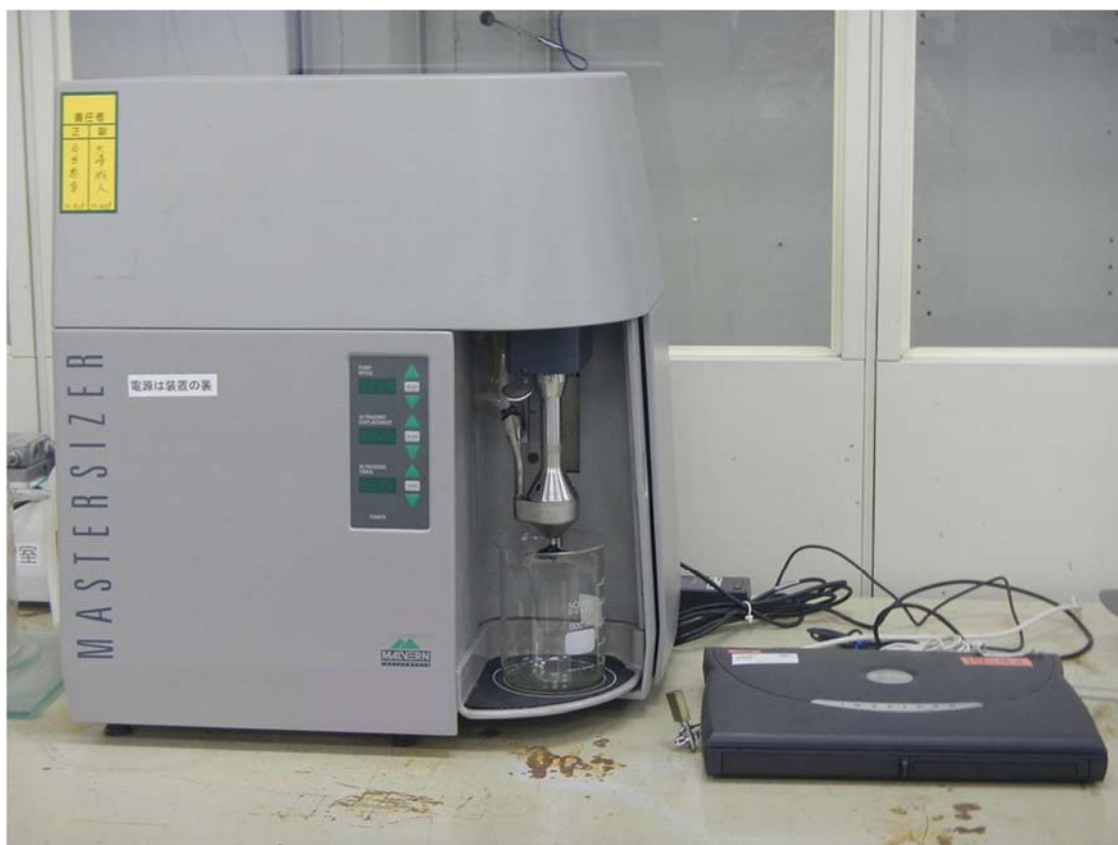
Figure 3.1-7 Laser diffraction particle size analyzer (Malvern/MASTERSIZER Micro)
