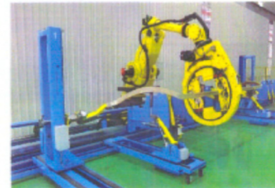
Gen Stator Coil taping machine
