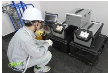
High Performance Monitoring System 5 componets analyzer (NO x , SO 2 , CO, CO 2 , O 2 )
