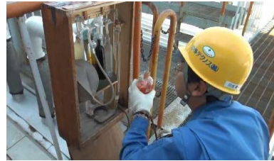
CO 2 , O 2 and N 2 Measurement by Orsat
