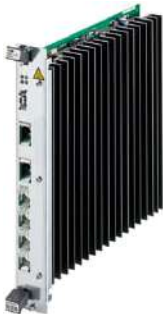
CESM3 148+ Gbps switching 4 x 1 GbE OR 4 x 10 GbE Uplink Core Unit
