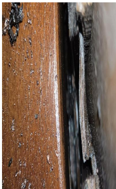
Burnt marks observed on Transformer
