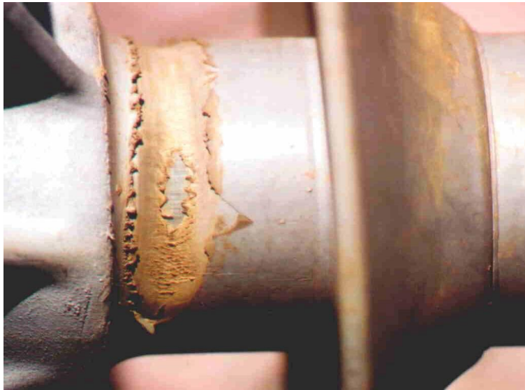
Sheath damage due to rope abrasion
