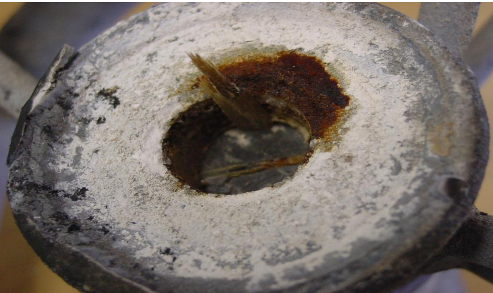
Initial (a) and subsequent (b) damage of a line post core subjected to excessive bending load
