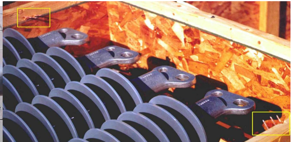
Nails protruding from a crate can lead to insulator damage
