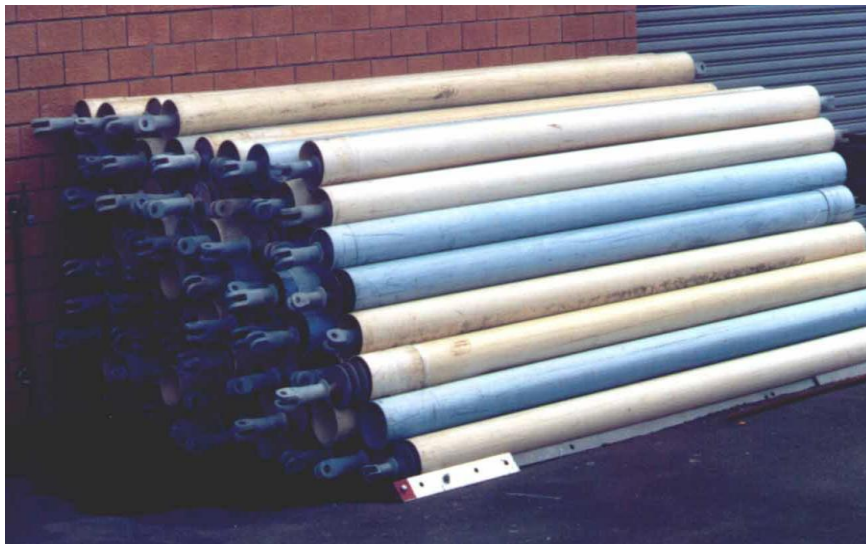
Insulators stored in plastic pipes
