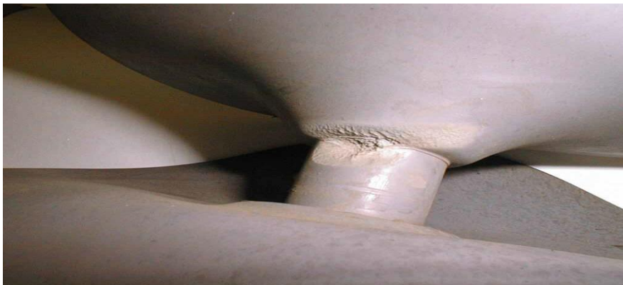
Housing damage from lifting line
