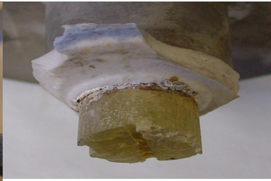
Initial (a) and subsequent (b) damage of a line post core subjected to excessive bending load
