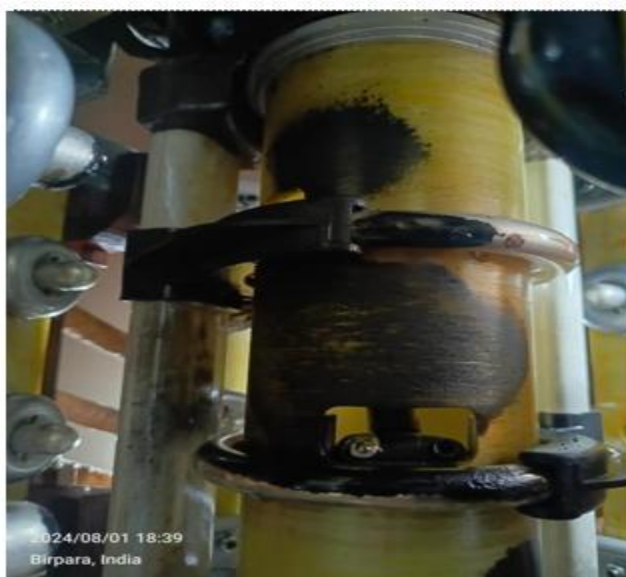
Flash mark on Y-Ph OLTC selector switch
