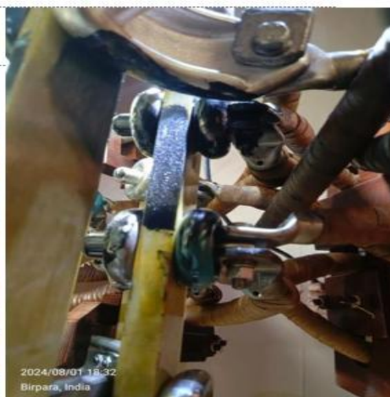
Flash mark on Y-Ph OLTC selector switch
