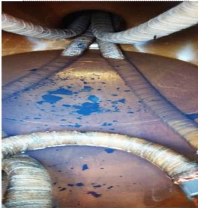
Carbon & burnt paper on Star winding Y1 Bushing winding lead take-out area
