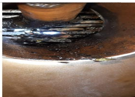
Damage at HV take-off point Y-Ph winding.
