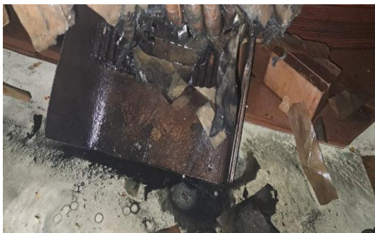
Flashover between B-phase tap lead and tank bottom
