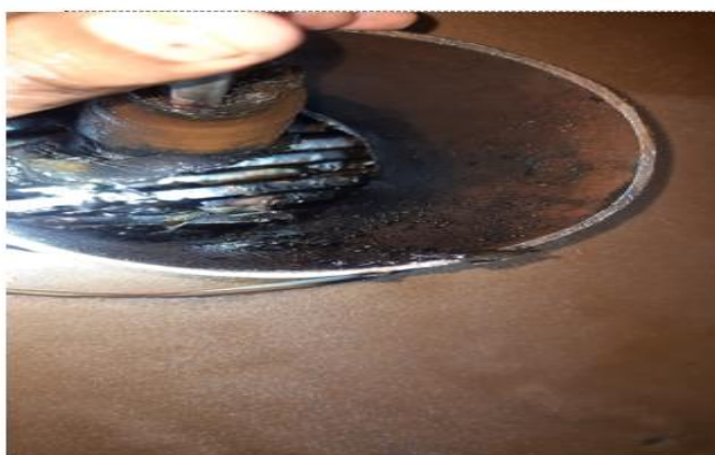
Damage at HV take-off point Y-Ph winding.
