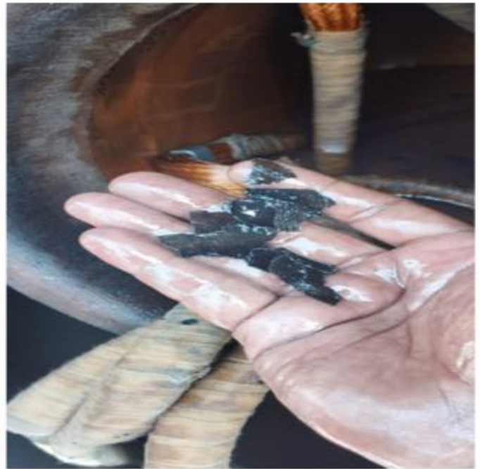
Carbon & burnt paper on Star winding Y1 Bushing winding lead take-out area
