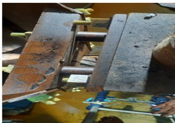
Carbon powder on lead exit support
