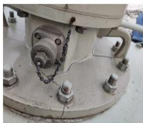
Crack observed on HV Bushings Flange
