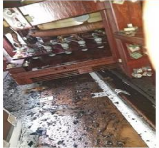
Burn Marks on Insulations Paper Carbon deposition observed on all over the active part
